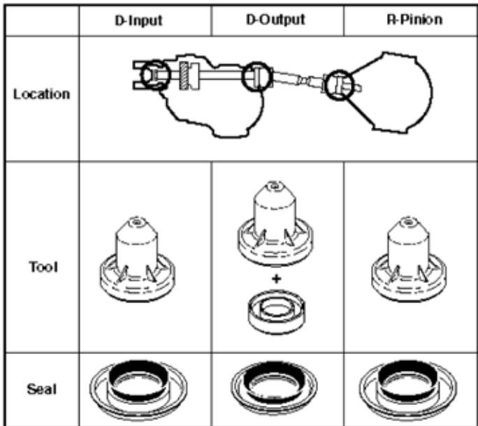
Pictured are the seal locations and typical Dana seal installation tools. The Dana 404 tandem drive axle tools are shown in this picture.
