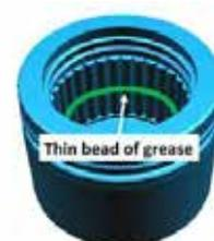
**\* Inspections must be performed at each maintenance interval to check for wear, damage, or looseness that could affect lubricant life and lead to driveline failure.**
